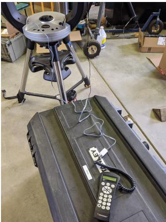
The grey cable you see here is an extension cable that was loose in the new box of stuff. The white block connects the hand controller to the extension cable and the other end goes in the port on the base of the telescope that is labeled "hand controller". I find it nice to have the controller next to the telescope especially for centering and guiding.
