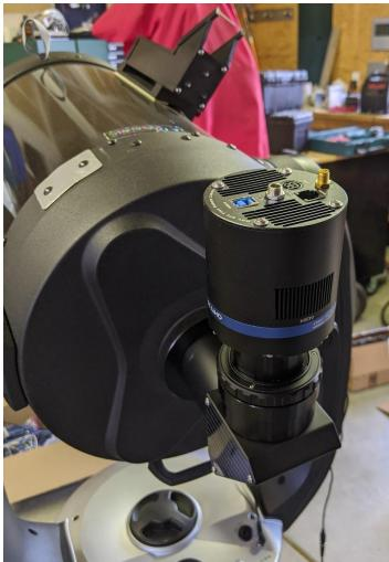
Next we connect the power to the camera. You will use the long cord with a barrel on one end and the lighter plug on the other that you used to use on the telescope. This goes into the camera after tying off to the handle like you are used to doing.
