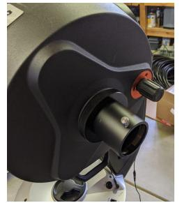
The visual back will thread directly onto the back of the telescope (after removing the cover on the back of the telescope). You want this to be tightened reasonably snug but it's not important to make it super tight.
