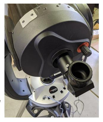
The next part will be to insert the camera into the diagonal on the exposed end you see here. Unlike the old camera, this setup cannot slide in so far that it will hit the mirror.
