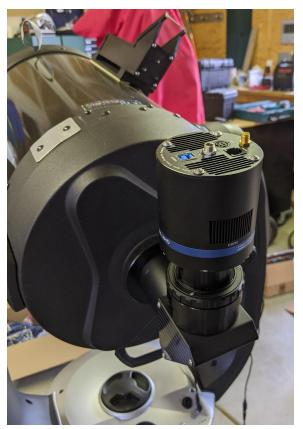
The camera assembly has a focal reducer already attached. I recommend leaving it on at all times and there room for it to be stored this way in the camera storage box that you've already seen. There is a ledge on the focal reducer that is about 25 mm back from the front. I like to align this ledge with the outer edge of the diagonal and this is where it should be clamped into place. If you push it in too far you may not be able to clamp it in place.
