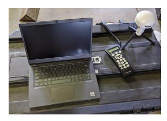
Everything is powered on here, including the telescope. You see the UT date and time and a nice picture on the laptop screen. Note that you should leave the laptop configured to use and show UT time.
