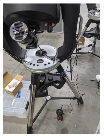
This image shows the power cable setup connected to the telescope and the QHY camera. You can see the power supply on the ground (it can also be placed on the tripod tray if you like). Also notice the cable has been tied off to the handle on the right fork arm. Finally, the right angle connector has been inserted into the CPC-1100 telescope and the other straight-male-barrel connector has been inserted into the power input in the center back of the QHY camera.
